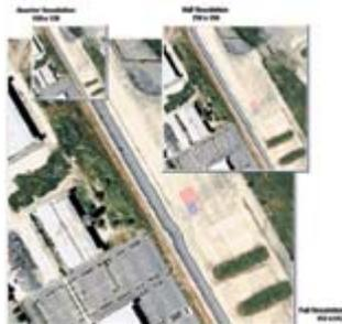
Figure 1. Because the JPEG 2000 wavelet-based technique encodes an image at multiple resolution levels (comparable to pyramid-based schemes but without the file-size overhead) a JP2 image can be decoded in different ways such as at full resolution half resolution and quarter resolution.
