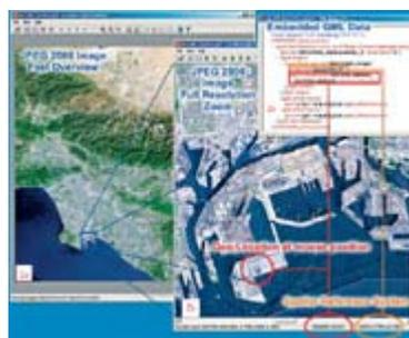
Figure 2a-2c. A screenshot of LuraTech LuraWave JP2 GeoView product demonstrating a fast overview of the whole large image (2a) a fast zoom-in on one region (2b) and a box showing GML code embedded in a JPEG 2000 file including GML coordinates corresponding to the cursor position (2c).
